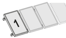
Fastening of the first collector in the row
